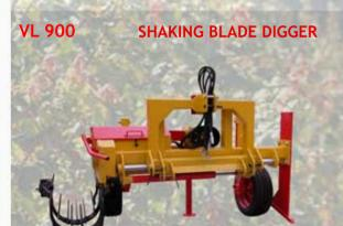
The **VL900** has a smooth operation thanks to the shaker which is operating in the opposite direction of the blade.
